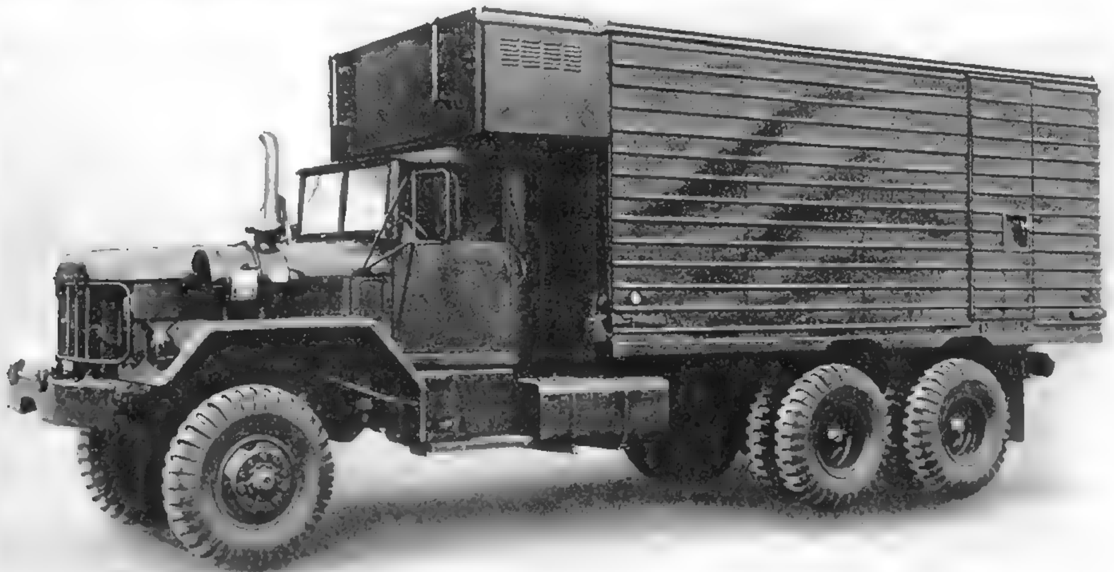
The M820A1 lacked the windows and air conditioner of the M820, but was equipped with heaters. (Photo courtesy of AM General)
